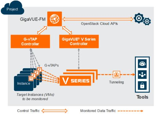
A G-vTAP Agent is deployed by installing the agent in the virtual instances. When a G-vTAP Agent is installed, a G-vTAP Controller must be configured in your environment. A G-vTAP Controller orchestrates the flow of mirrored traffic from G-vTAP Agents to the GigaVUE V Series nodes. A single G-vTAP Controller can manage up to 100 G-vTAP Agents deployed in the cloud.
