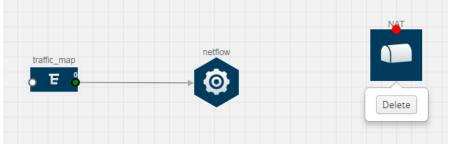
2. Drag and drop a link from the NetFlow application to a NAT device. A Link quick view is displayed. It is a header transformation operation that lets you configure the IPv4 destination IP of the NetFlow collector.
