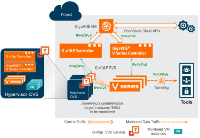
The G-vTAP Agents are deployed on the target hypervisors and the configuration file is to be modified based on the requirements and service. GigaVUE-FM connects to G-vTAP Controller and each G-vTAP Controller can talk to G-vTAP Agents. GigaVUE-FM receives the list of interfaces that can be used as the source or destination for the mirroring interface selected in GigaVUE-FM. GigaVUE-FM mirrors and forwards the traffic to the V Series nodes based on the deployed Monitoring Session.
